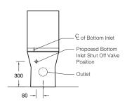
Vario pan connector S-trap installation
